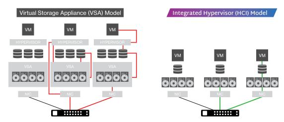
By virtue of having a tight integration between hypervisor, hardware, and storage, Scale Computing has created a hypervisor-embedded storage architecture within HC3 to deliver high efficiency along with streamlined simplicity. This unique architecture provides a number of benefits.
